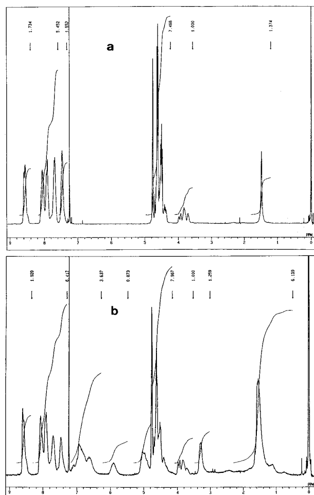
Figure 13 ^1\text{H-NMR} spectra of the polymer resulting from the reaction of PEPB and DBA with solvent \text{CDCl}_3 at 60^\circ\text{C} : (a) PEPB, and (b) after 3 h at 250^\circ\text{C} .
